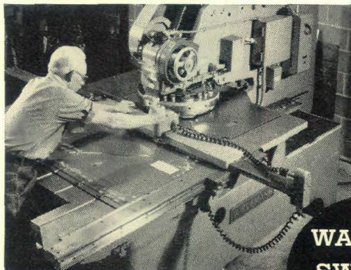
*Production-line speed, accuracy and costs are obtained in short-run production with the turret punch presses made by the Wiedemann Division of Warner & Swasey.*
