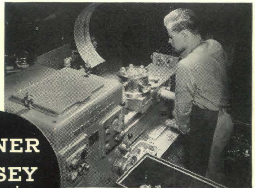
Warner & Swasey Electrocycle® Lathe producing brass valve bodies.
