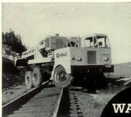
Railroad Gradall drives right over track on maintenance-of-way work. Gradall is a registered trade name.
